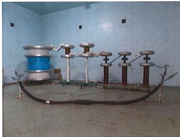
G2: 样品局部放电试验及交流耐压试验 Partial discharge test and AC voltage test on the sample
