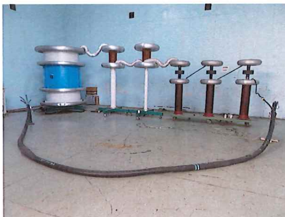
C2: 样品交流电压试验 AC voltage test on the sample
